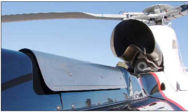
Because of its higher exhaust gas temperature, the AS350B3 sports a stainless steel shield on the tail boom to protect the aluminum structure. The shield is the easy way to tell the B3 from its predecessors.
