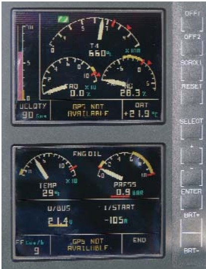
(Above) On the AS350B3, power gauges have been replaced by a vehicle and engine management display—a sophisticated flat panel unit that displays a single-needle gauge called a first limit indicator that combines the 3 limiting engine parameters into the single needle, simplifying power management for the pilot. (Below) The center console offers a new style, cooler operating push switch for system controls and lights.
