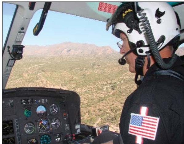
McClendon flies a speed data point demonstrating the 130-KIAS-plus cruise of the AS350B3. Note airspeed indicator.
