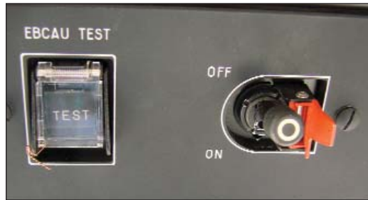
After several variants of FADEC switch configuration, Eurocopter has settled on a single guarded switch mounted overhead in the latest B3s.
