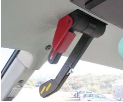
Rotor brake and fuel shutoff levers have been moved from the floor to the overhead position in the AS350B3 for easier pilot access.
