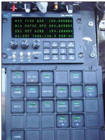
(Above) On the AS350B3, power gauges have been replaced by a vehicle and engine management display—a sophisticated flat panel unit that displays a single-needle gauge called a first limit indicator that combines the 3 limiting engine parameters into the single needle, simplifying power management for the pilot. (Below) The center console offers a new style, cooler operating push switch for system controls and lights.
